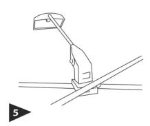
OPTIONAL Attach lights to top of frame by sliding the plastic X Blocks under the frames cross sections.
