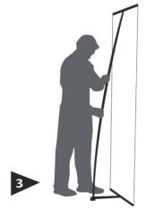
Flex pole and insert bottom of pole into the hole of metal foot base.
