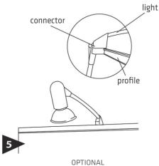
To attach light, place into top of pole connector.
