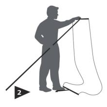
Assemble pole. Attach top pole connector to top profile of graphic.
