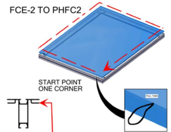
Install graphic by pressing the FCE-2 into the channels of PHFC2 extrusion. To pull graphics out of the channels, use tabs on the front side
