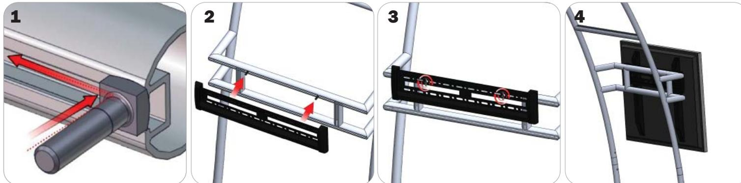
Locate all components needed to assemble the monitor mount with the TRI-30MM Channel Tube Connection method. You will need (1) monitor bracket, (2) Square Bolts, and (2) Wingnuts.
