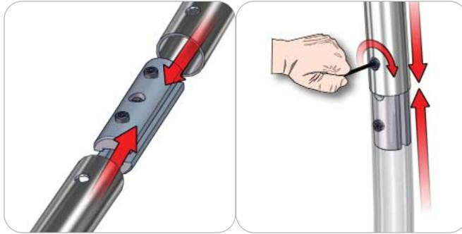
Compress the unlocked connector and slide one tube onto each end. Lock both screws carefully using your allen key tool. Be sure to lock securely, but do not overtighten.
