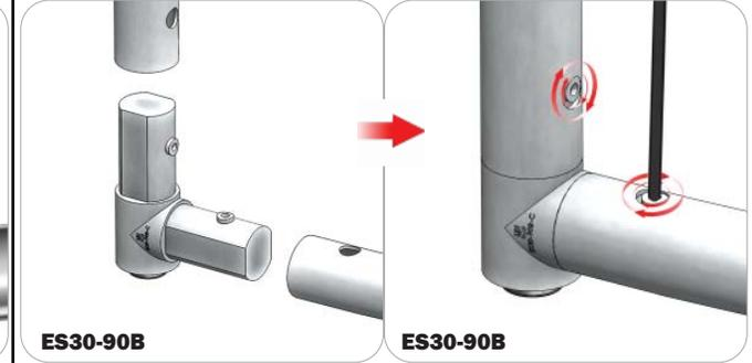
Compress one unlocked end of the connector and slide it through one tube end. Compress the other end of the connector and slide the second tube on. Lock both screws carefully using your allen key tool. Be sure to lock securely, but do not overtighten.
