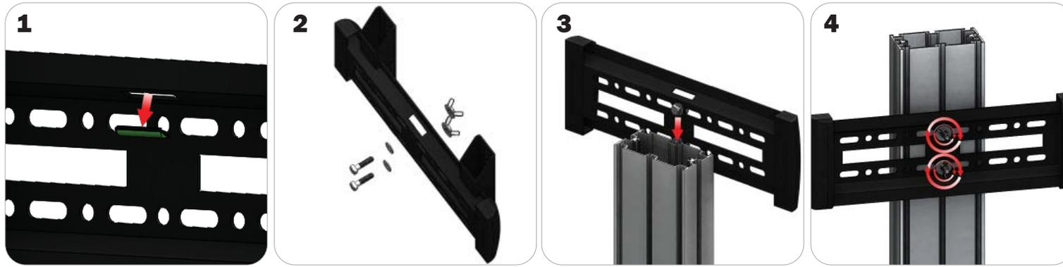
Locate all components needed to assemble the monitor mount with the channel connection A method. You will need (1) monitor bracket, (2) square head bolts, (2) washers, and (2) wingnuts.
