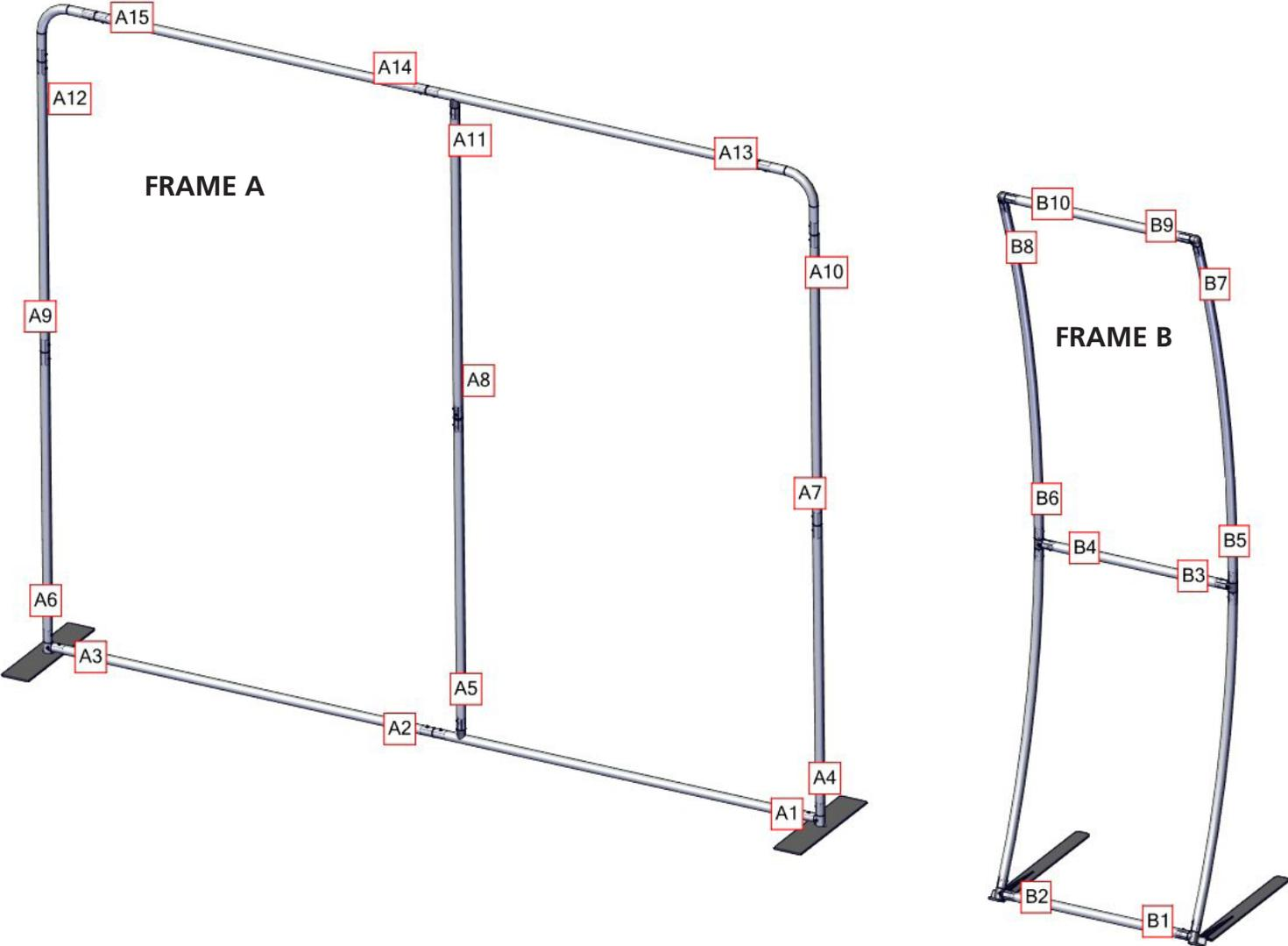
Frame A and B stand independently of one another, no connection hardware required.
