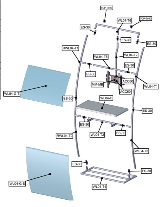
WL04 Frame Assembly: Assemble unit by laying tubes flat on the floor. Connect the tube rails following the labels by matching number to number. See detailed drawing.
