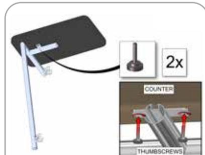
Install counter to mounting tube with 8/32" thumb screws, repeat for second screw.
