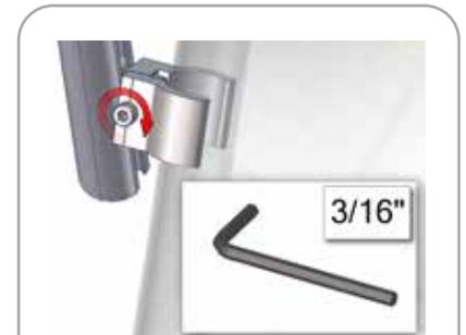
Secure second tube clamp TC-30 around backwall and tighten with 3/16" hex key tool.
