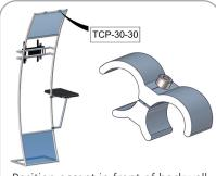
Position accent in front of backwall in desired location. Secure tube clamp at top of frame.
