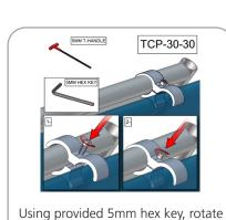
bolt clockwise to secure accent to top of fabric backwall.
